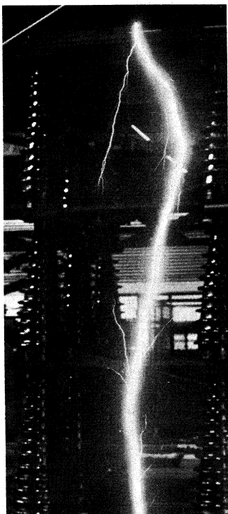
BY COURTESY OF GENERAL ELECTRIC COMPANY ARTIFICIAL LIGHTNING PRODUCED IN A LABORATORY BY A DISCHARGE OF ABOUT 2,000,000 V.
