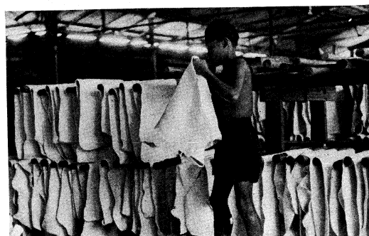
Hanging sheets of rubber to dry in a processing plant at Medan, Sumatra
